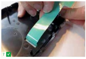
Make sure that the tail of the membrane switch foil pulled neatly through the housing.
