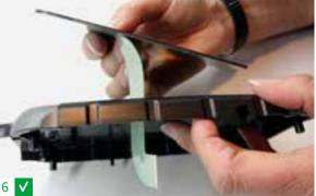
Push the tail of the membrane switch foil carefully through the designated groove.
