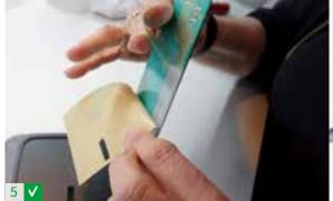
Grab the tail of the PCB in between two fingers. Then proceed to remove the protective layer from the sticky layer (backside). **Please note:** Do not touch the membrane switch foil while performing this step!
