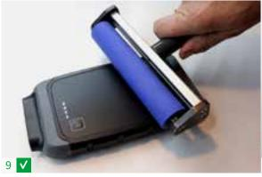
Press the backside plate down and roll over it so it attaches well to the adhesive foil.
