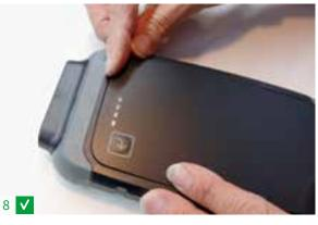
Carefully place the backside over the housing.
